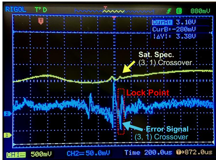
Figure 3.6: Probe's scope trace of the saturation absorption signal (yellow) used to generate the error signal (blue) to lock the laser to a specific signal. Despite the noise seen on the trace, linewidth measured using heterodyne detection was measured to be within a few MHz [89].
