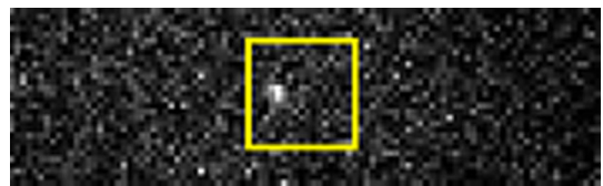
FIG. 1 (color online). Fluorescent image of a single atom acquired with a CCD camera. The field of view of the single photon counter is shown as a yellow square.
